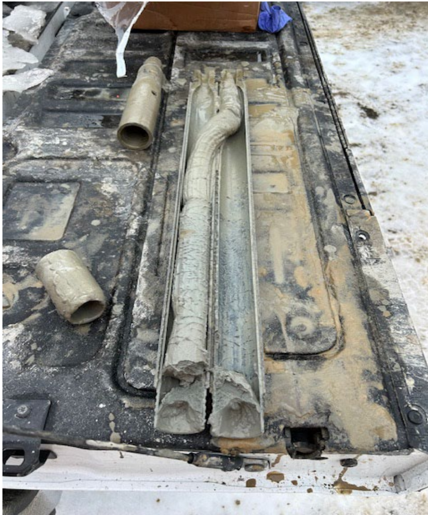
Gray silty clay sample common to all boreholes. Soft to firm in consistency
