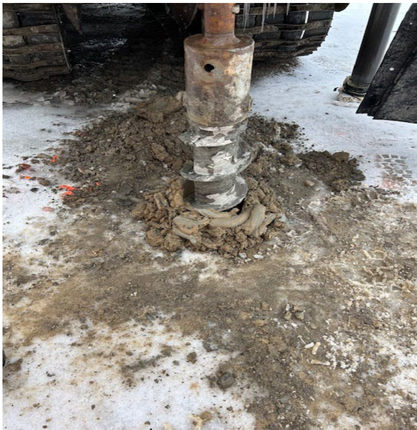
Photo #8-BH-04 Silty Clay-soft to firm
