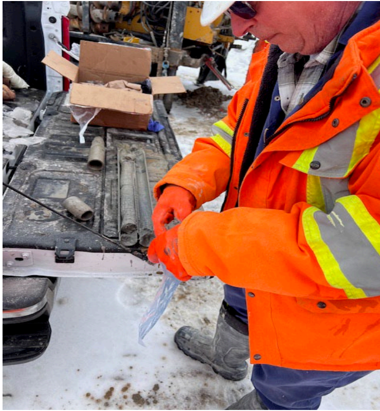
Photo #9 – Silty clay SS in BH-05. SPT (N) = 0. Wt. of hammer
